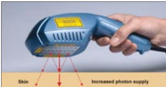
Standard probe with photon reflection foil
